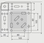
For wheels and castors Ø 160 mm and Ø 200 mm With screw-on plate 80 x 105 mm
